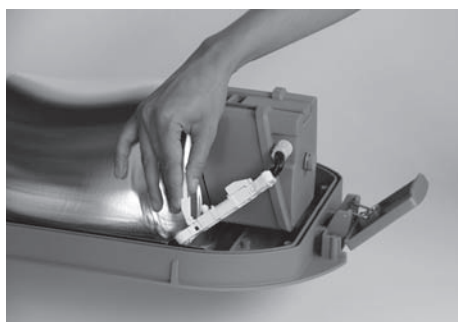
4 Connector latch release
